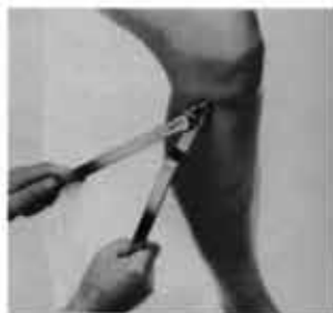
Cutter for cutting off KIRSCHNER wires, Tibia head screws, bolts, pins, up to 3 mm diam.
